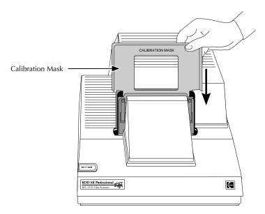
E. Click OK. The Scanner will then display several messages. As prompted, wait for calibration to complete, reinsert the appropriate film holder — with film in place — and wait while focusing occurs and your image appears in the Driver window.
